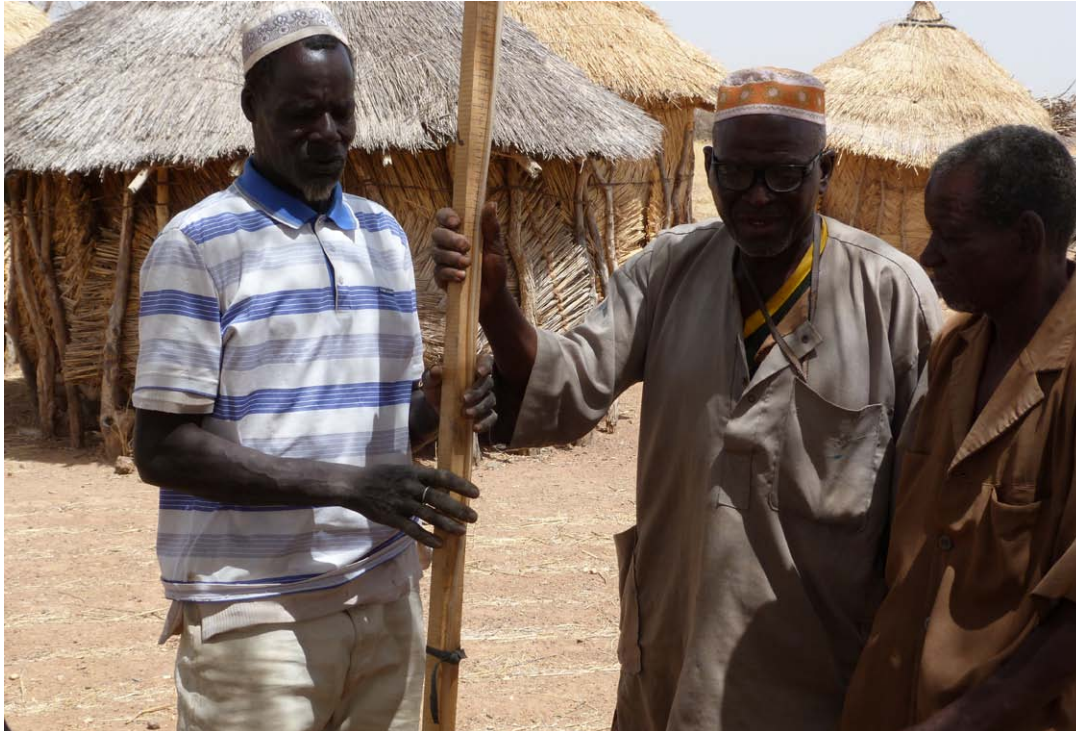
Demonstration of a water-level gauge for determining elevation contours in the PATECORE village of Kolokoum. The technique learned more than 20 years ago is still used today © T. Jenisch
