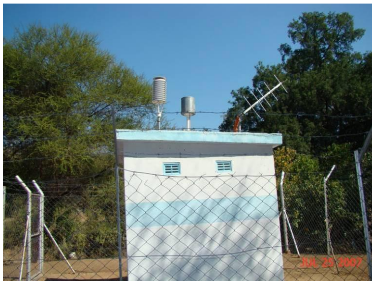
Figure A4.1: A typical DCP shelter with air temperature/ humidity sensor, rain gauge and antenna on roof.
