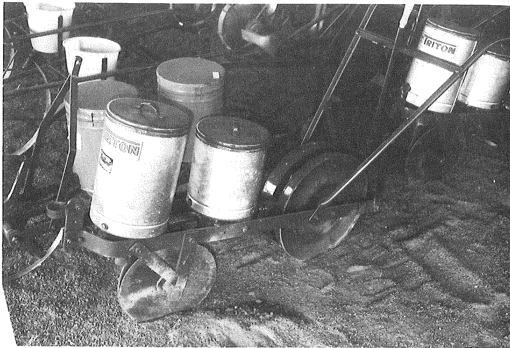
Fig. E 55: Triton seeder with double disc shares, Brazil (Photo: Schmitz)
