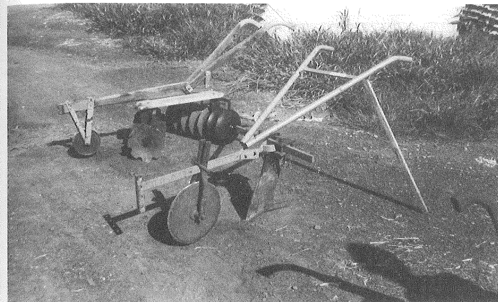
Fig. E 30: Chisel plow with a single tool in Brazil (in the foreground) (Photo: IAPAR)
