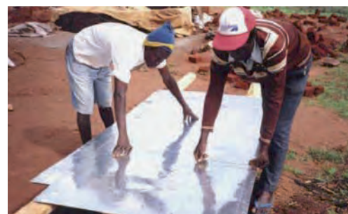
Manufacturing square-sectioned gutters from galvanized plain iron: shaping them with a piece of wood (Nissen-Petersen, 2007).
