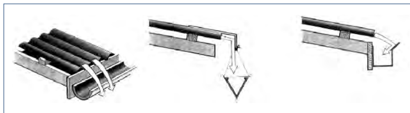
Water overshooting the gutter (left) and options to avoid water overflows (Skinner, 2003 in Doyle, 2008).
