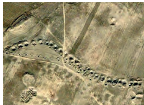
Aerial view of a qanat system in Iran with the access shafts forming a trail towards a village. (www.livius.org)
