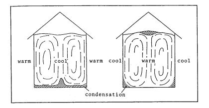
Condensation occurs particularly in silos, but also in warehouses, mainly close to the walls and roofs from where it drops down onto the stored produce. Sometimes it is also found under the tarpaulins of stacked commodities.
