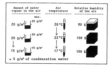
Condensation occurs in stores primarily when there are great differences in the temperatures inside and outside the store. A typical example is when the outside walls become hotter or colder (temperature fluctuations between day and night).
