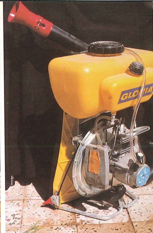
For bigger areas an engine-driven portable sprayer is more economical.
