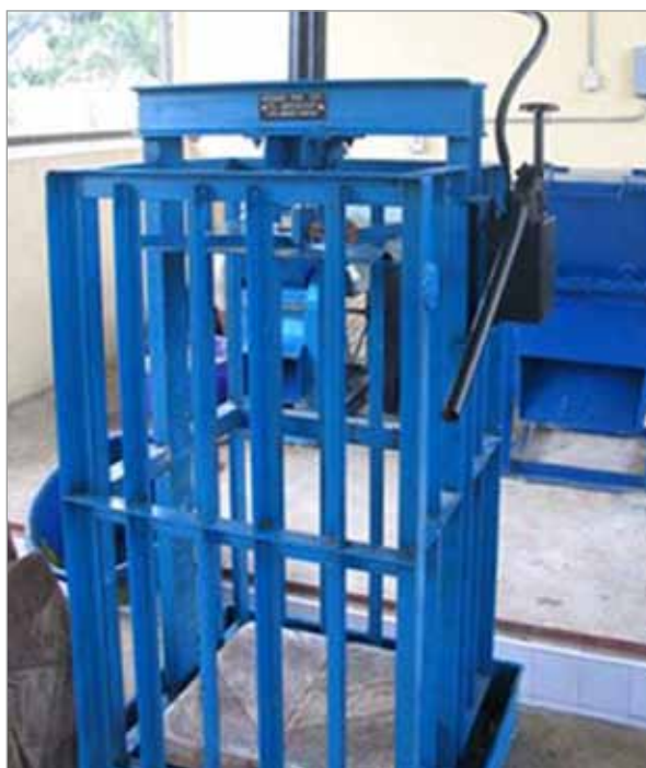
Figure 35: Hydraulic cassava press 39
