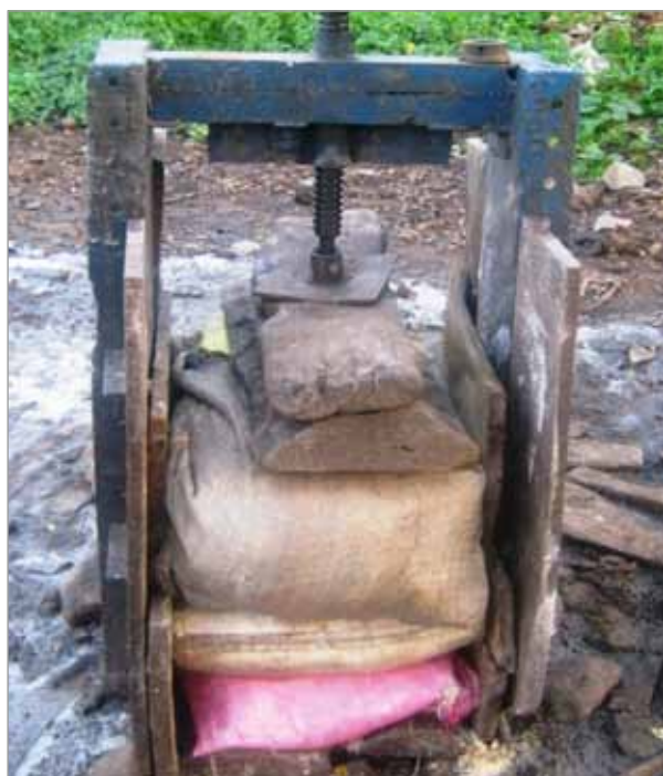
Figure 34: Screw cassava press 39
